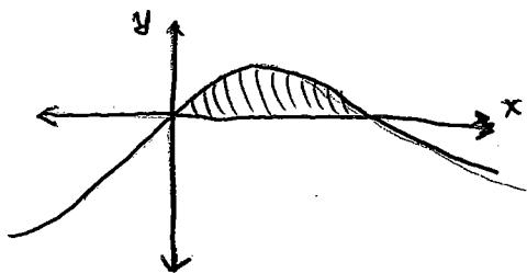
$$\text{Area} = \int_{x=0}^{x=2} y \, dx = \int_{t=0}^{t=1} (t - t^2)(3t^2 + 1) \, dt \quad (\text{since } dx = (3t^2 + 1)dt)$$
