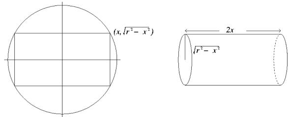
Using  $V = \pi R^2 H$  gives  $V(x) = 2\pi (r^2 - x^2)x = 2\pi r^2 x - 2\pi x^3$ ,  $0 \le x \le r$ . Since  $V'(x) = 2\pi r^2 - 6\pi x^2 = 2\pi (r^2 - 3x^2) = 0$  only when  $x = r/\sqrt{3}$ , the largest possible volume is  $V(r/\sqrt{3}) = \frac{4\pi r^3}{3\sqrt{3}}$ .
